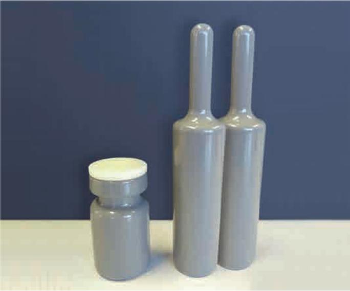
**Fig. 10:** Dummies – metal core with powder coating
