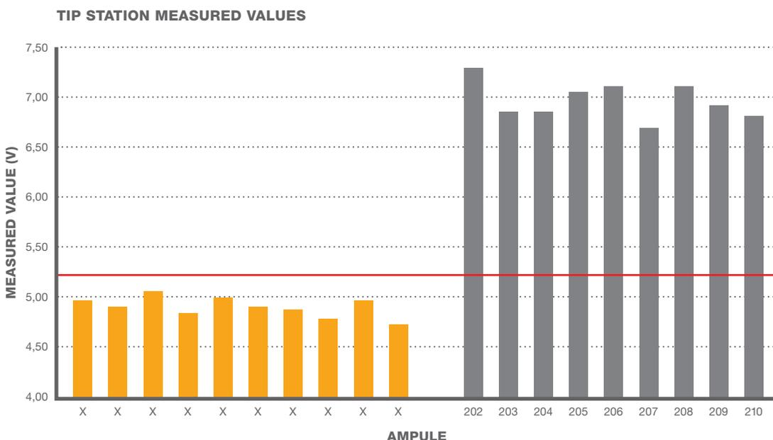
**Fig. 3:** Tip inspection - Measured values for good products (left) and bad products (right)
