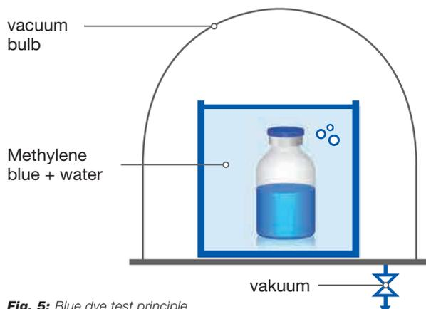
**Fig. 5:** Blue dye test principle
