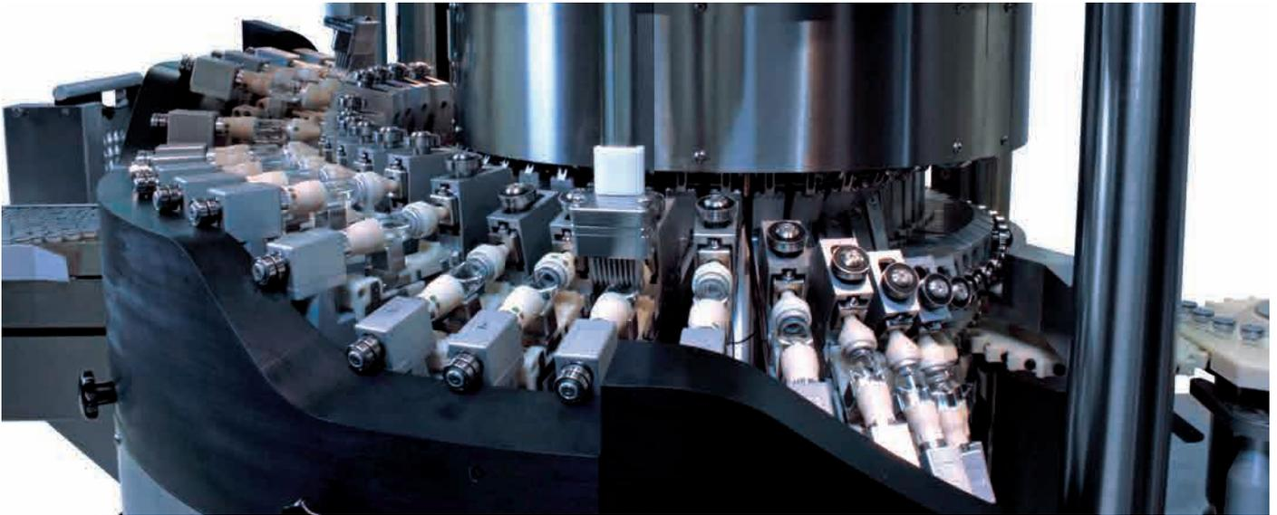
Fig. 1: Product transport, sidewall inspection
